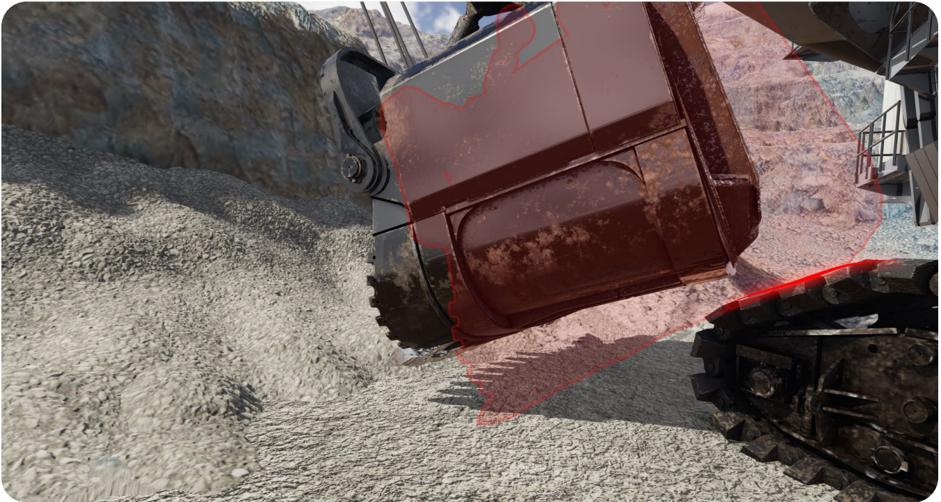
Dipper to crawler shoe contact can occur when digging in close proximity to the tracks and during the "return to tuck" part of the dig cycle
