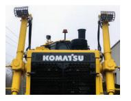
The two cab mounted lights have also been upgraded to LED.
