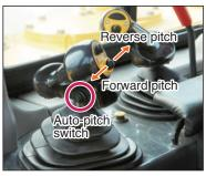
the pitch position from digging to dump position with no additional lever movements. The blade pitch control can be set through the monitor to automatically return to the digging position when reverse is selected.
