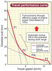
Lockup mechanism of torque converter is automatically actuated to transfer engine power directly to the transmission in usual dozing speed range. Locking up the torque converter eliminates loss of horsepower by 10%. Because the electronically controlled engine is extremely efficient, a decrease in fuel consumption is realized while also maintaining machine power.
