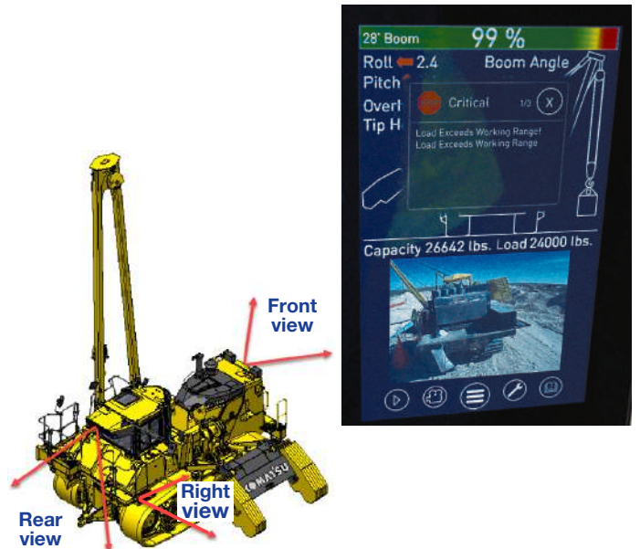
Three cameras provide additional views around the machine. Forward view camera (above), with selectable right-side camera and rearview camera are standard. Load Moment Indicator information is displayed at top of screen.
