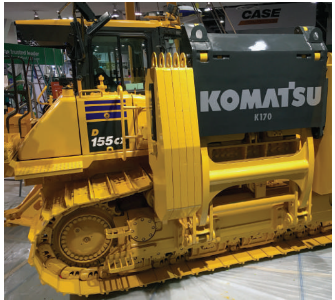
Steps, platform and handrails provide easy access to the fuel tank
