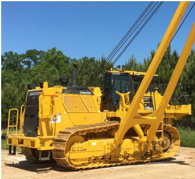
Steps and handrails on 4-corners of machine provide access for servicing the engine and other components
