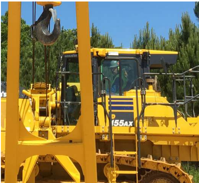
ROPS structure integrated into cab eliminates side posts
