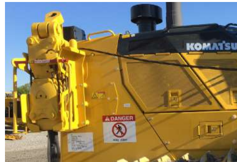
Bracket to store blocks during shipping is standard
