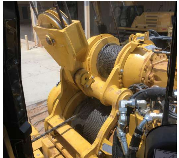
Good view to winch drums for spooling
