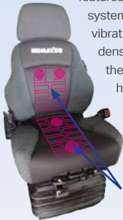
Heater and ventilator
