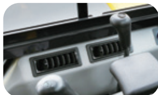
Heater with fresh air vents
