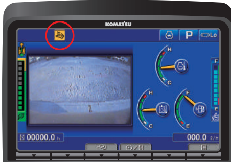
Soot level indicator
