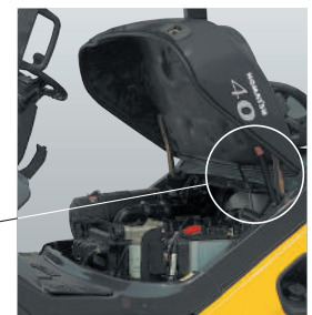
Locking engine hood provides protection while servicing
