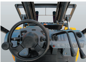
Finger-tip operation with the electric F/R lever
