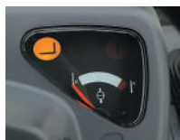
KOPS Plus Hydraulic Lock Indicator
