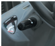
Finger-tip operation with the electric F/R lever
