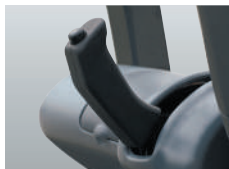
A double acting type brake lever prevents mishandling
