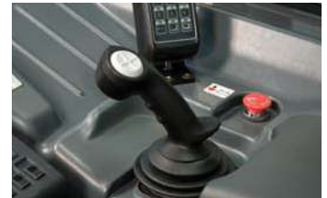
An ergonomically designed multi-function control handle offers easy and intuitive control of truck drive and hydraulic functions.
