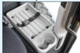
Engine shutdown secondary switch
