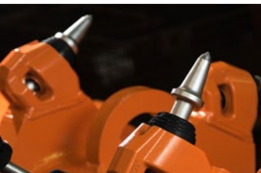
The JS series bit holder features a rear access hole for easy bit removal saving time and energy. The induction case-hardened bore provides extended life of the bit blocks through multiple sleeve change-outs. Lower profile helps alleviate potential wear that can shorten the life of the block.
