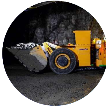
Underground hard rock WX04B load haul dump and charger
