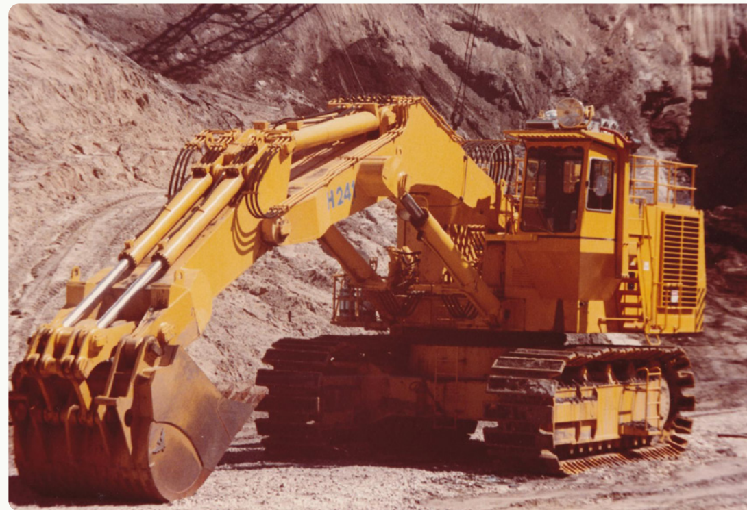
History of electrification: H241, first electric-driven hydraulic mining excavator globally
