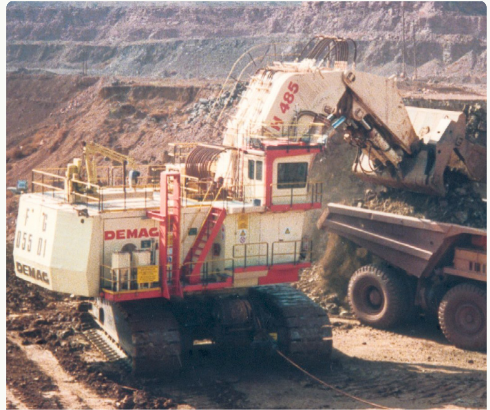
History of electrification: H485, the largest hydraulic mining excavator of its time powered by an electric motor
