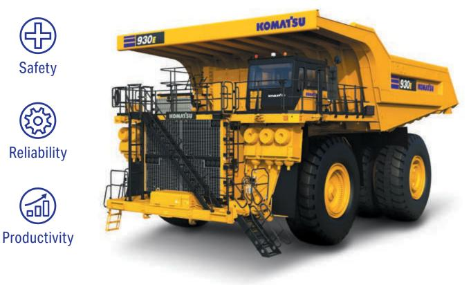
**Gross horsepower** 2 611 kW (3,500 HP) **Nominal GVW** 521 631 kg (1,150,000 lbs.)
