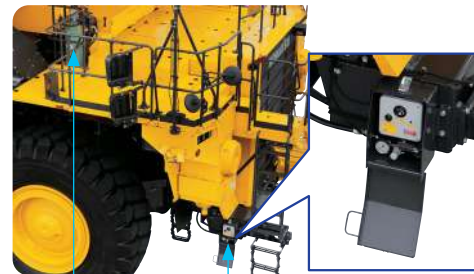
Grease pump and reservoir Refill port
