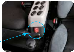
Secondary engine shutdown switch
