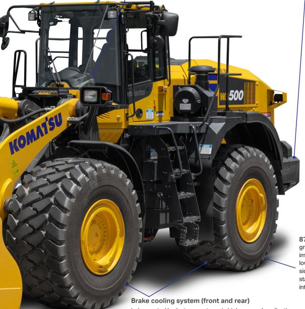
875/65 tires increase ground contact area for improved stability. The low profile also reduces sidewall flex for more stability while dumping into trucks or hoppers.
