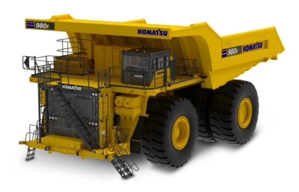
**Gross horsepower** 3 281 kW (4,400 HP)
